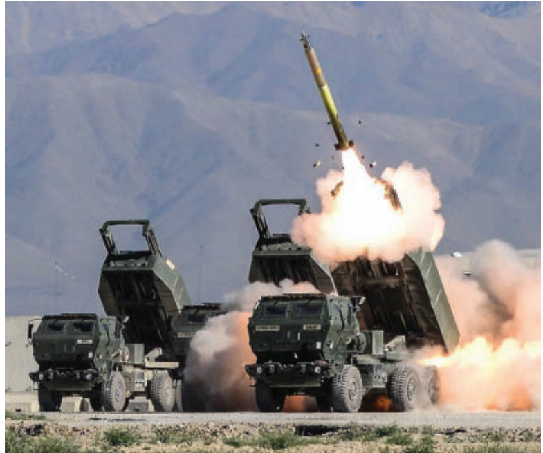
The High Mobility Artillery Rocket Systems (HIMARS) will fire the Army's future long-range Precision Strike Missile (PrSM), as well as other kinds of munitions at ranges from 43 to 250 miles.
