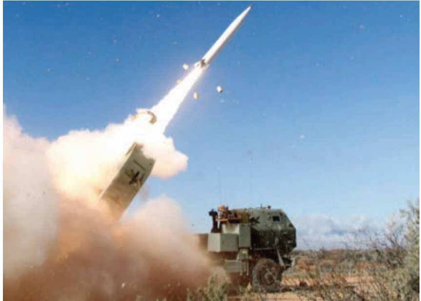
The PrSM missile has the ability to home-in on radio signals from enemy radar or communications to refine its targeting before impact.
