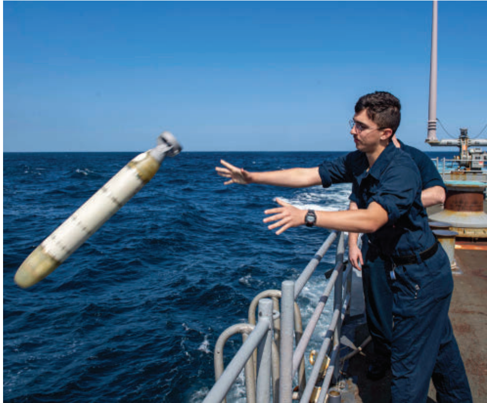
The MK 39 Mod 2 expendable mobile antisubmarine warfare training targets (EMATT) mimic the sounds and behavior of enemy submarines for anti-submarine warfare training.
